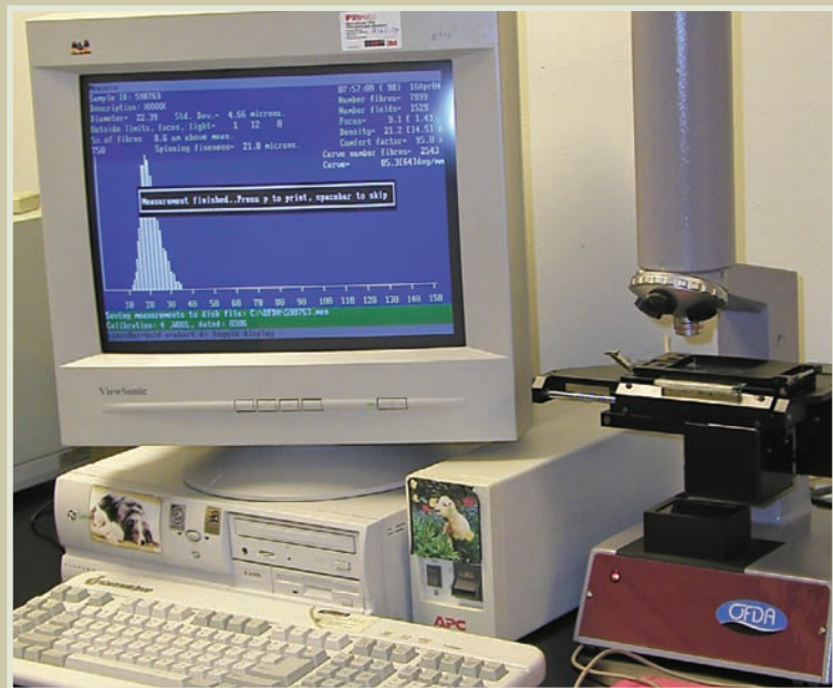
OFDA100 software analyzes fiber images and derives AFD, SD, and CV measurement of 2000 to 4000 longitudinal fiber sections. OFDA100 also measures curvature and medullation.
