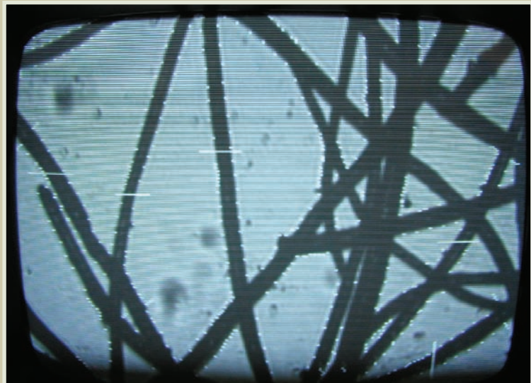
OFDA100 software analyzes fiber images and derives measurement of diameter of a large number of longitudinal fiber sections.
