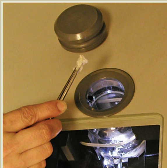
Sample cups of fiber snippets for individual animal fiber diameter testing by Sirolan LaserScan instrument.
