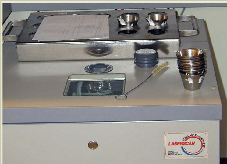
Sample cups of fiber snippets for individual animal fiber diameter testing by Sirolan LaserScan instrument.
